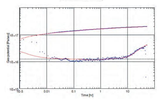
Figure 4.6 Log-log Plot of Pressure and Pressure Derivative of C2 Sand
