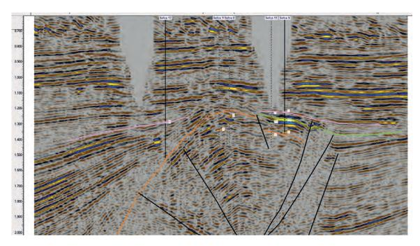
Figure 3.4 Seismic line BO327-80 showing Selva Level B North and South Prospects
