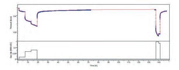
Figure 4.8 Pressure and Gas Rate of C2 Sand
