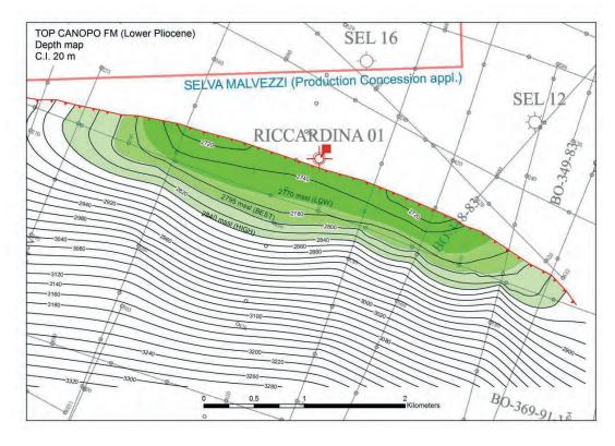
Figure 3.11 Riccardina Prospect; PVO depth structure map at top Canopo Formation (metres subsea)
