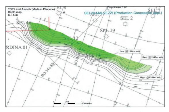
Figure 3.7 Level A South Prospect, Depth Structure Map showing Low, Mid and High Case contacts
