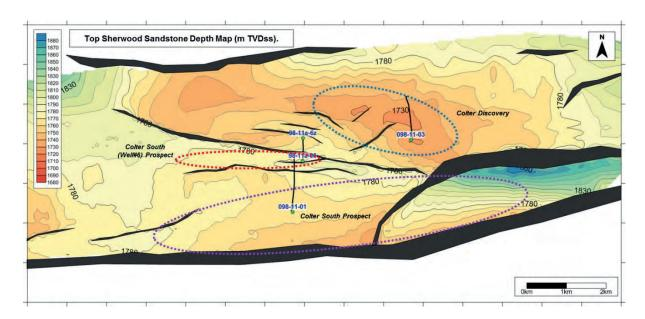
Figure 2.9: Well Locations and Corallian's Top Sherwood Sandstone Depth Map (m TVDss) (Top Sherwood Sandstone penetration in each of the wells is shown by the green dot. The dashed coloured ellipses highlight the locations of the Colter Discovery, Colter South prospect and Colter South (Well#6) prospect.)
