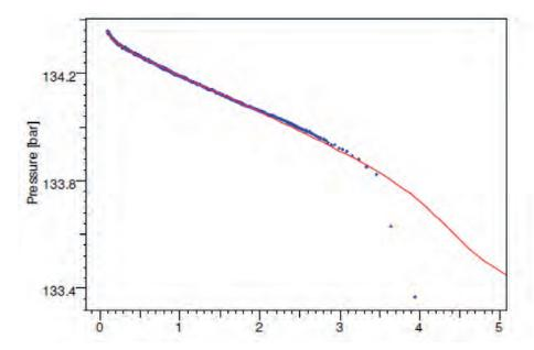
Figure 4.7 Horner Plot of C2 Sand
