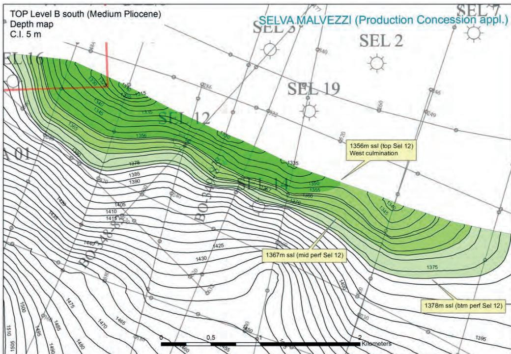
Figure 3.6 Level B South Prospect, Depth Structure Map showing Low, Mid and High Case contacts
