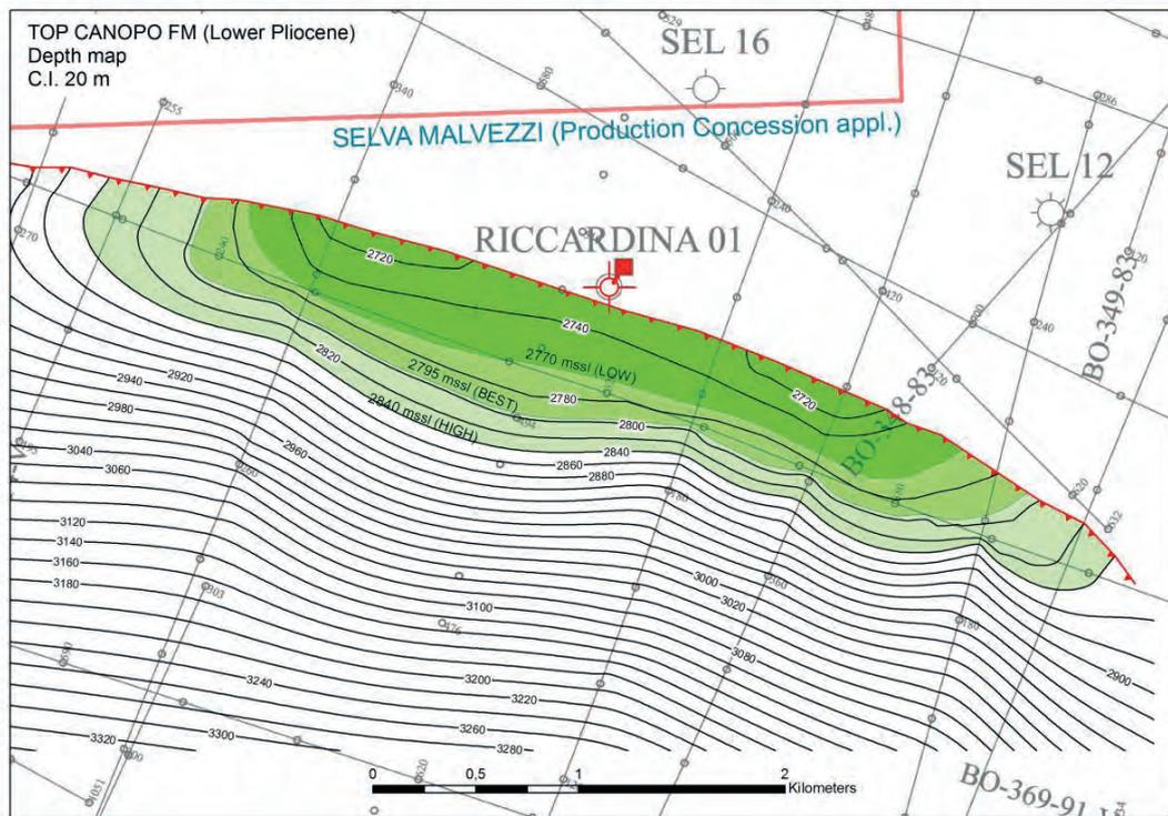
Figure 3.11 Riccardina Prospect; PVO depth structure map at top Canopo Formation (metres subsea)
