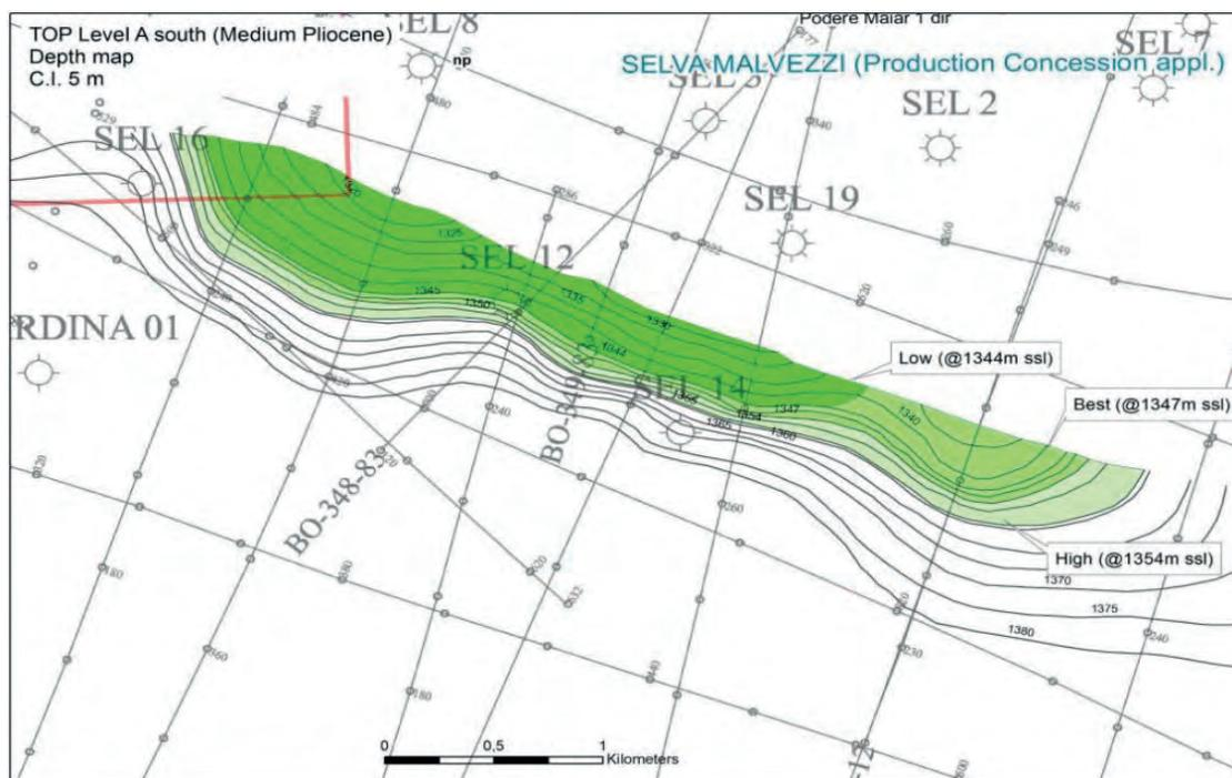
Figure 3.7 Level A South Prospect, Depth Structure Map showing Low, Mid and High Case contacts
