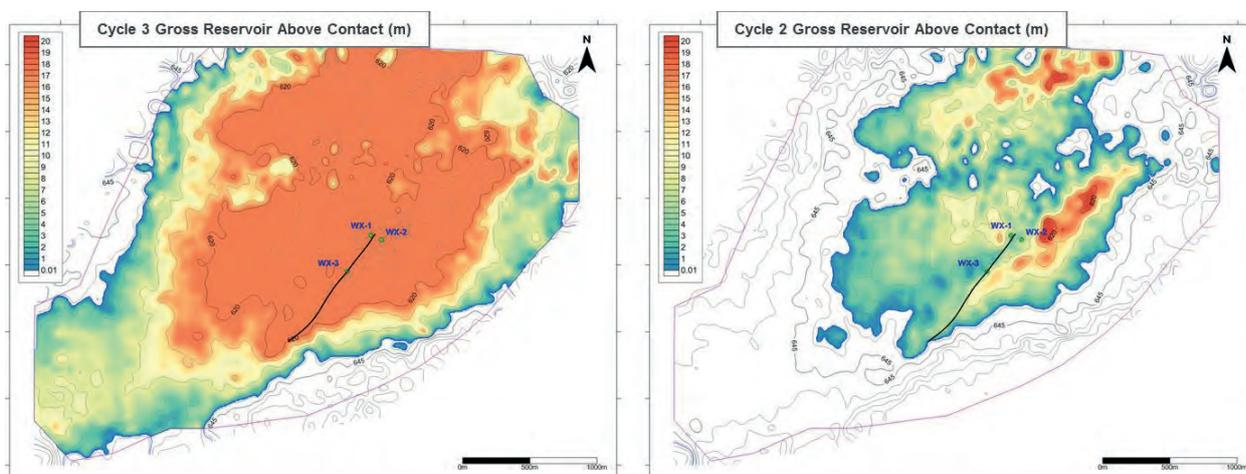
**Figure 2.7: Gross Reservoir Thickness Above OWC – Mid Case**
