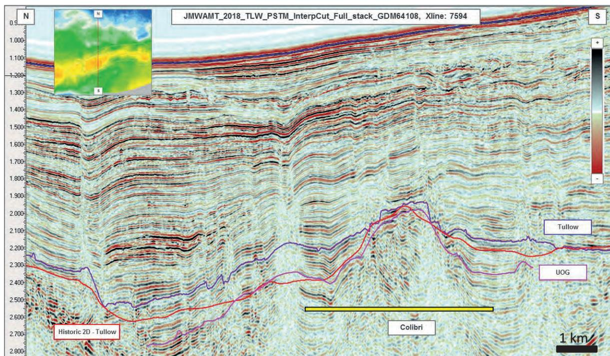
Figure 3.8: S-N Seismic Section Over the Colibri Prospect
