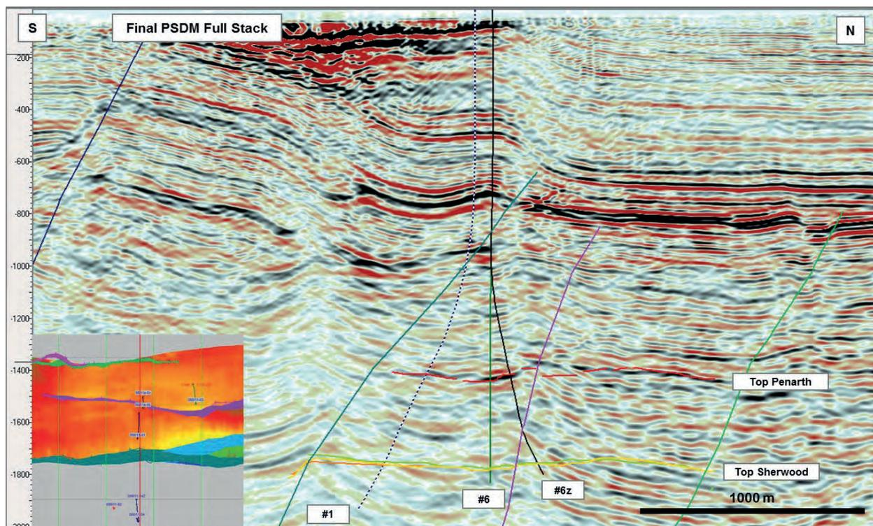
**Figure 2.10: S-N Seismic Section through Wells 98/11-1, 11a-6 & 11a-6z**
