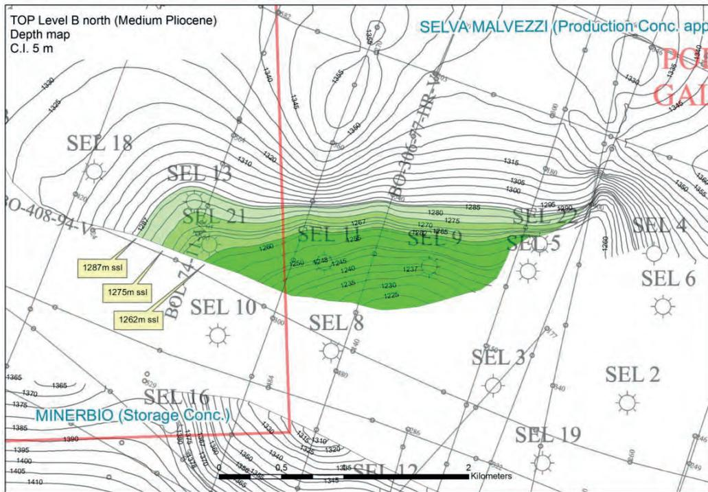
Figure 3.5 Level B North Prospect, Depth Structure Map showing Low, Mid and High Case contacts
