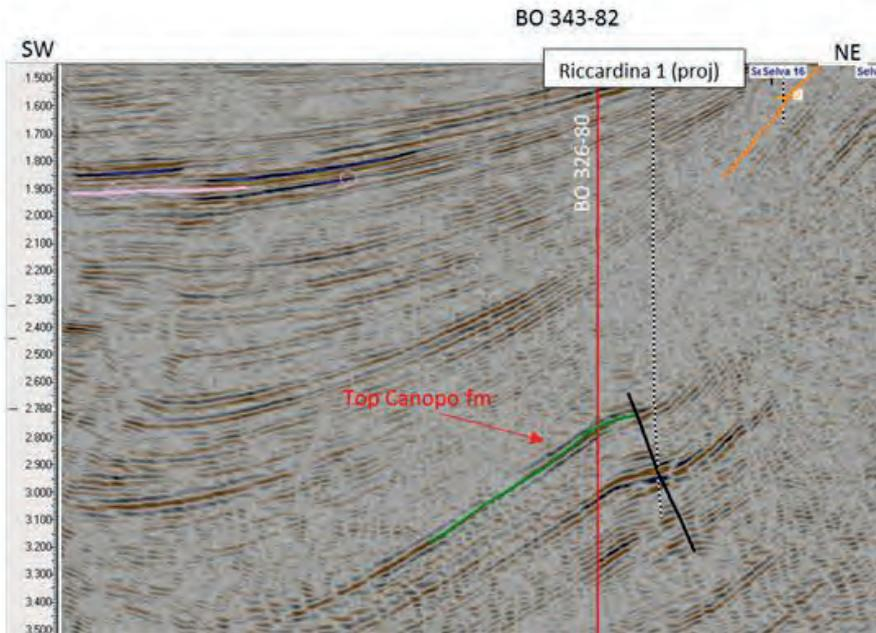
Figure 3.10 Riccardina Prospect: Seismic Line BO343-82 shows gas prospect in Canopo Formation
