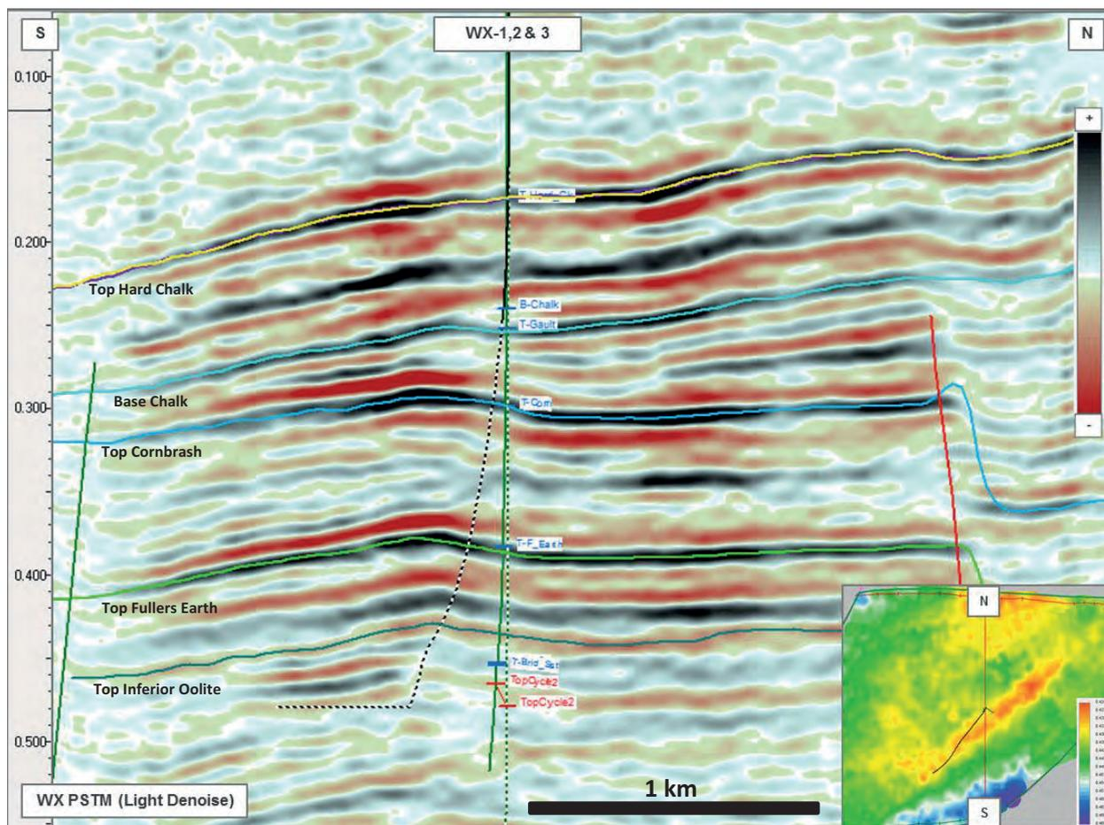
Figure 2.3: N-S Seismic Line Through the Waddock Cross Field
