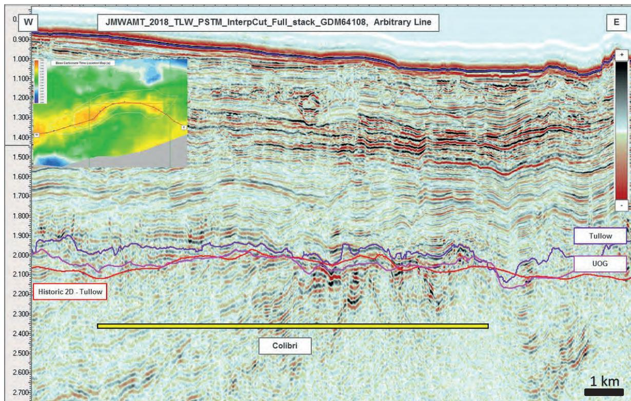
Figure 3.7: W-E Seismic Section Over the Colibri Prospect
