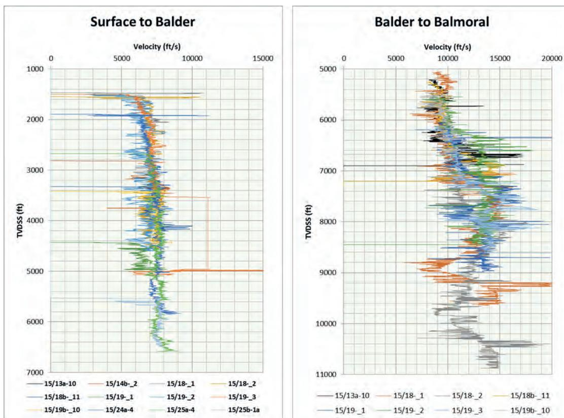
Figure 2.18: Sonic log velocities from proximal well control
