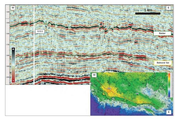
Figure 2.16: Arbitrary seismic line from running West to East along the crest of the Crown discovery
