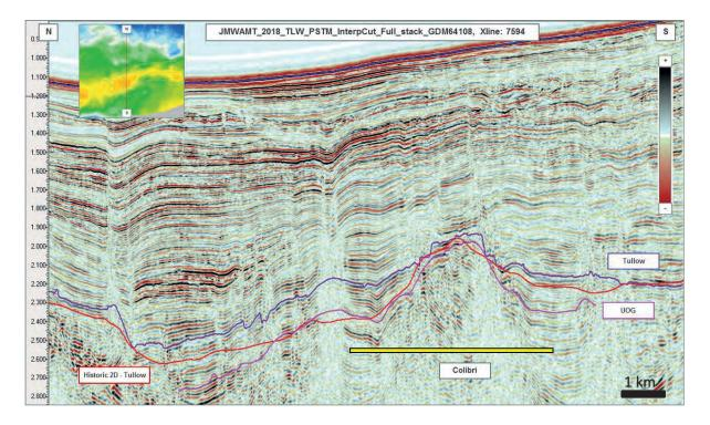
Figure 3.13: S-N Seismic Section Over the Colibri Prospect
