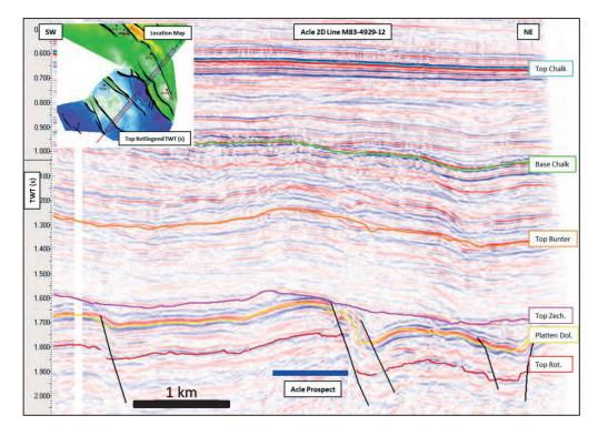
Figure 3.6: 2D Seismic Line across Acle Prospect
