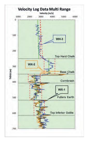
Figure 2.4: Log Velocity Plot - Waddock Cross Velocity Model (Waddock Cross-1, 2 & Wareham-3)
