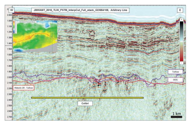
Figure 3.12: W-E Seismic Section Over the Colibri Prospect
