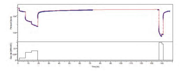
Figure 4.8 Pressure and Gas Rate of C2 Sand
