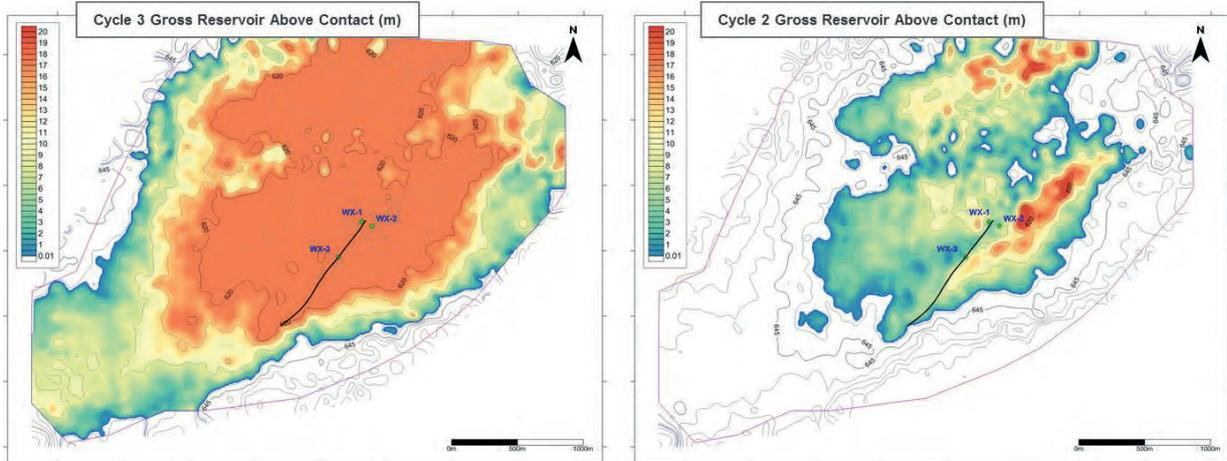
**Figure 2.7: Gross Reservoir Thickness Above OWC – Mid Case**
