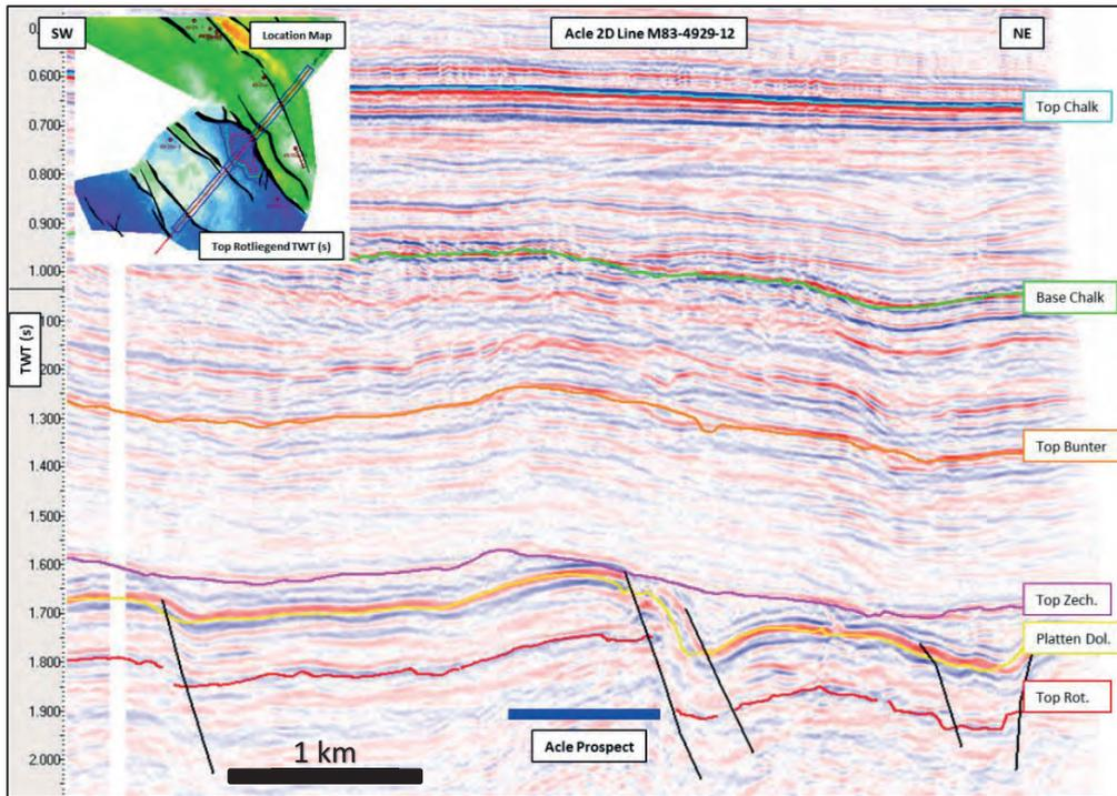
Figure 3.6: 2D Seismic Line across Acle Prospect
