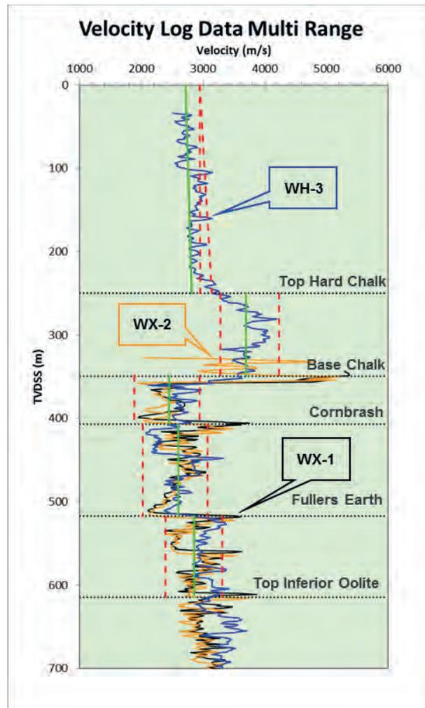
**Figure 2.4: Log Velocity Plot - Waddock Cross Velocity Model**
