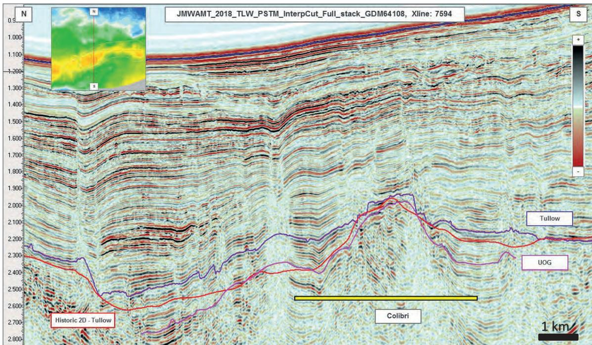
Figure 3.13: S-N Seismic Section Over the Colibri Prospect
