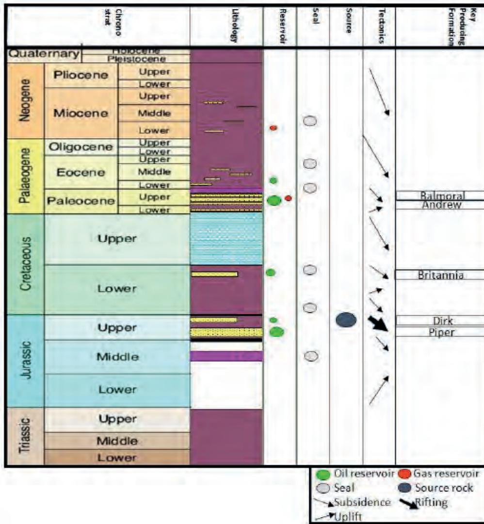
Figure 2.15: Stratigraphic Column, Witch Ground Graben and Fladen Spur.
